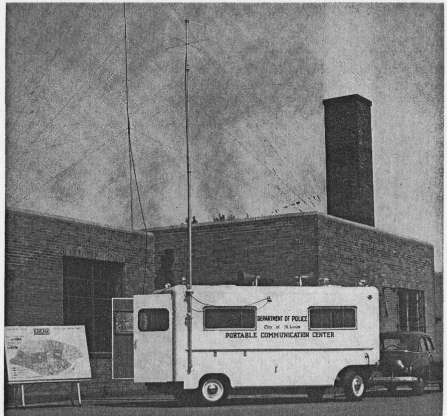
COMPLETE PORTABLE-MOBILE COMMUNICATIONS TRAILER in use by the St. Louis, Mo. PD. Although the trailer weighs 2500 pounds it can be towed by a car.
